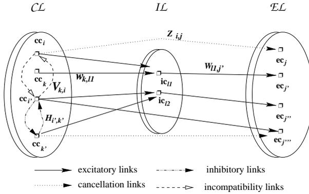
Fig. 2. The three-layered neural architecture for a causal problem.
