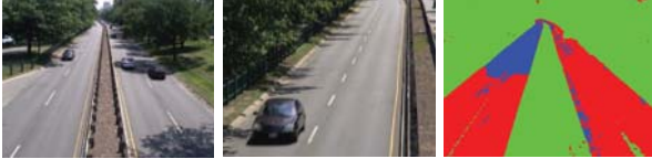
Fig. 5. From left to right : image from Camera 1, image from Camera 2 and the occlusion map obtained with our method. Green signifies no activity, red signifies region of activity as seen by Camera 1 only and blue signifies regions of activity seen by both cameras.
